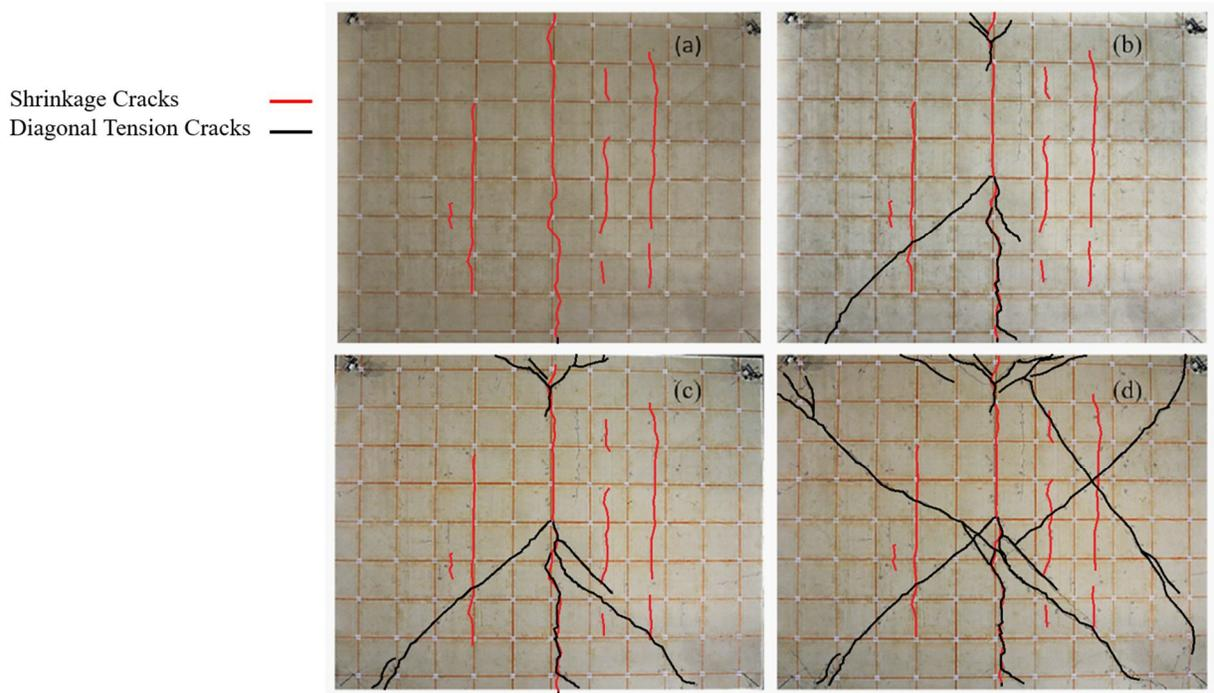
Figure 4. Progression of failure for specimen 3/6.25-4-L-NF-DT. (a) Before testing. (b) First appearance of diagonal tension cracking. (c) First appearance of diagonal tension cracking in opposite direction. (d) Crack pattern past failure
