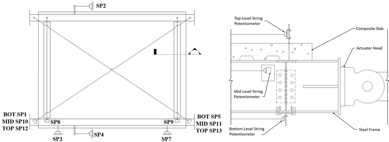
Figure 2. Instrumentation Setup for Cantilever Diaphragm Tests (a) Plan view. (b) Section.
