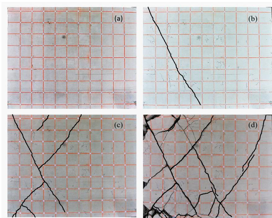
Figure 6. Progression of failure for specimen 3/7.5-4-N-NF-DT. (a) Before testing. (b) First appearance of diagonal tension cracking. (c) First appearance of diagonal tension cracking in opposite direction. (d) Crack pattern past failure
