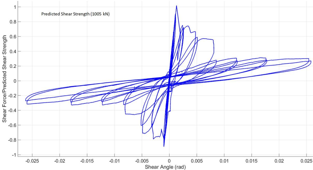
Figure 7. Load Deformation Plot of Specimen 3/7.5-4-N-NF-DT
