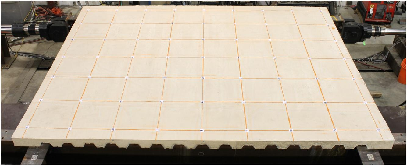
Figure 3. Experimental Setup for Cantilever Diaphragm Tests
