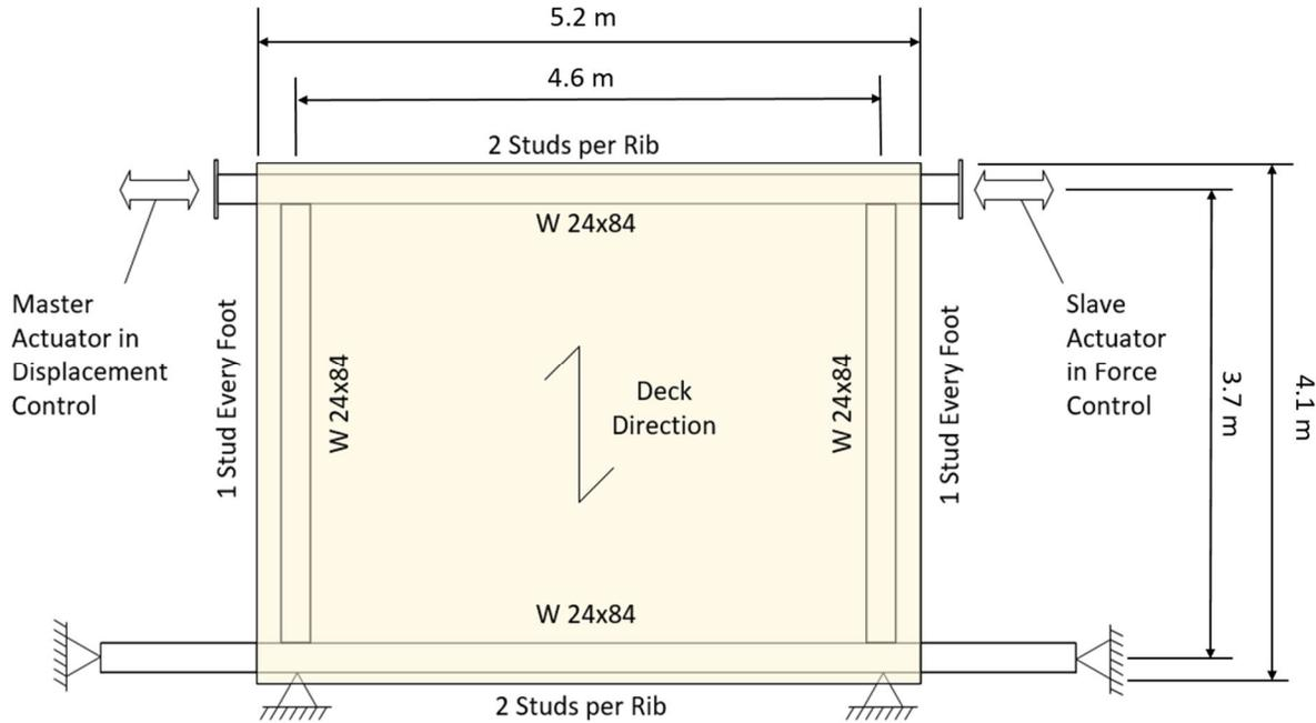
Figure 1. Experimental Setup for Cantilever Diaphragm Specimens
